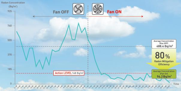
Radon Mitigation Efficiency by Ventilation
